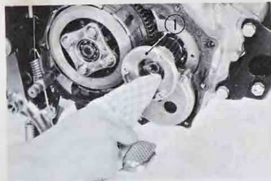
① Oil filter rotor
