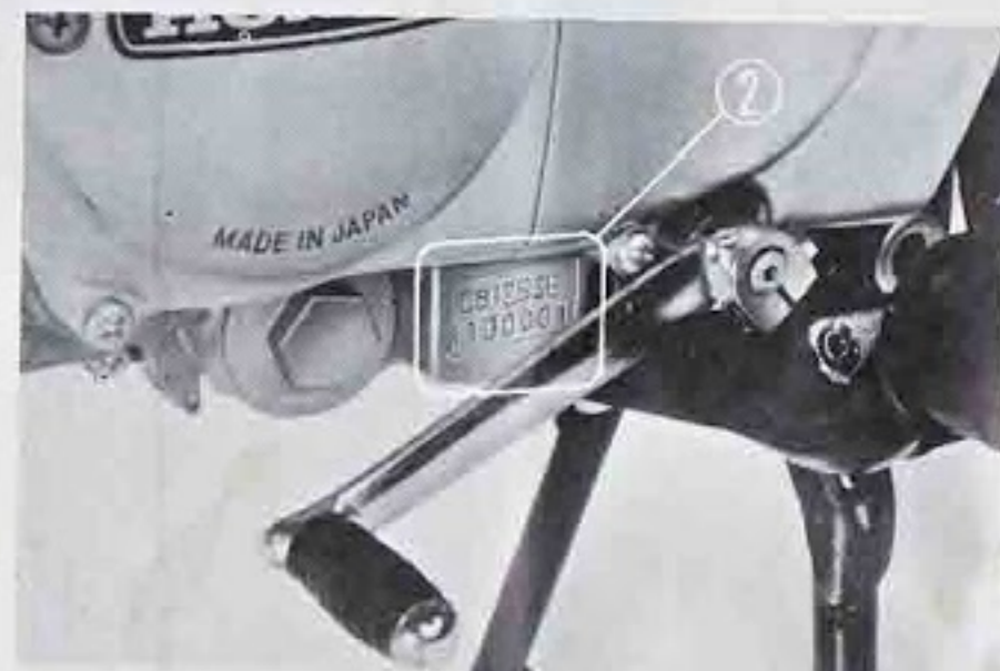
② Engine serial number
